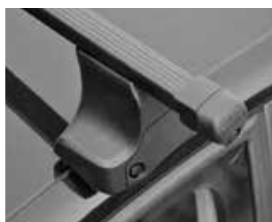
An example of a roof rack for motor cars without water channels.
